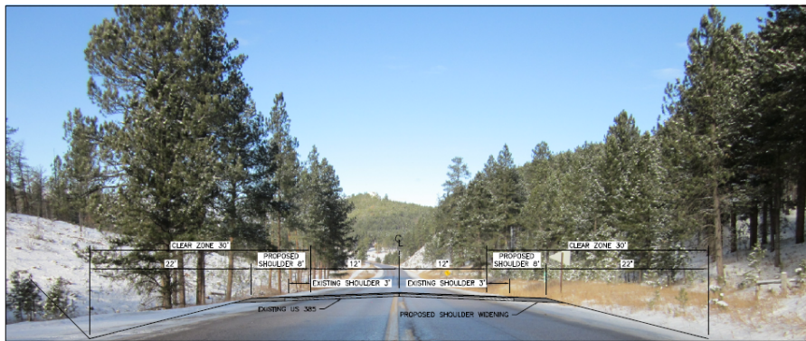
TYPICAL SECTION (SHOULDER WIDENING) MRM 96.657 TO MRM 102.37
