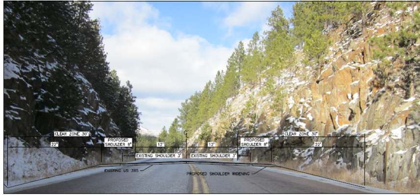
TYPICAL SECTION (SHOULDER WIDENING) MRM 87.2 TO MRM 96.657
