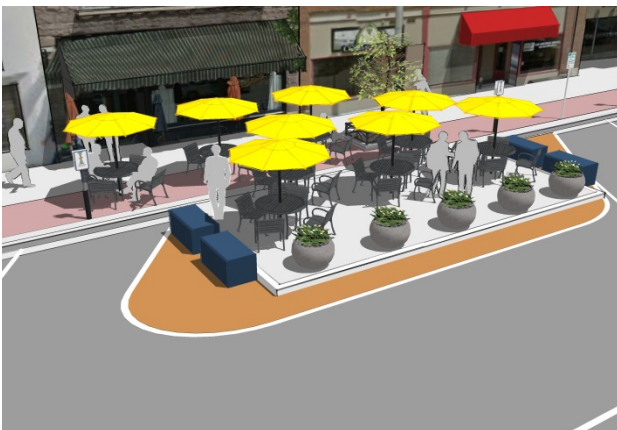
Painted curb extension in Sioux Falls, SD.
