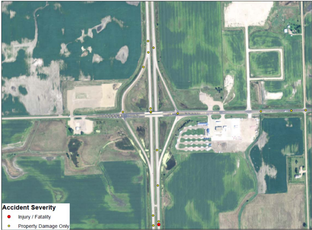
Figure 8: Crash Location & Severity 2009-2011
