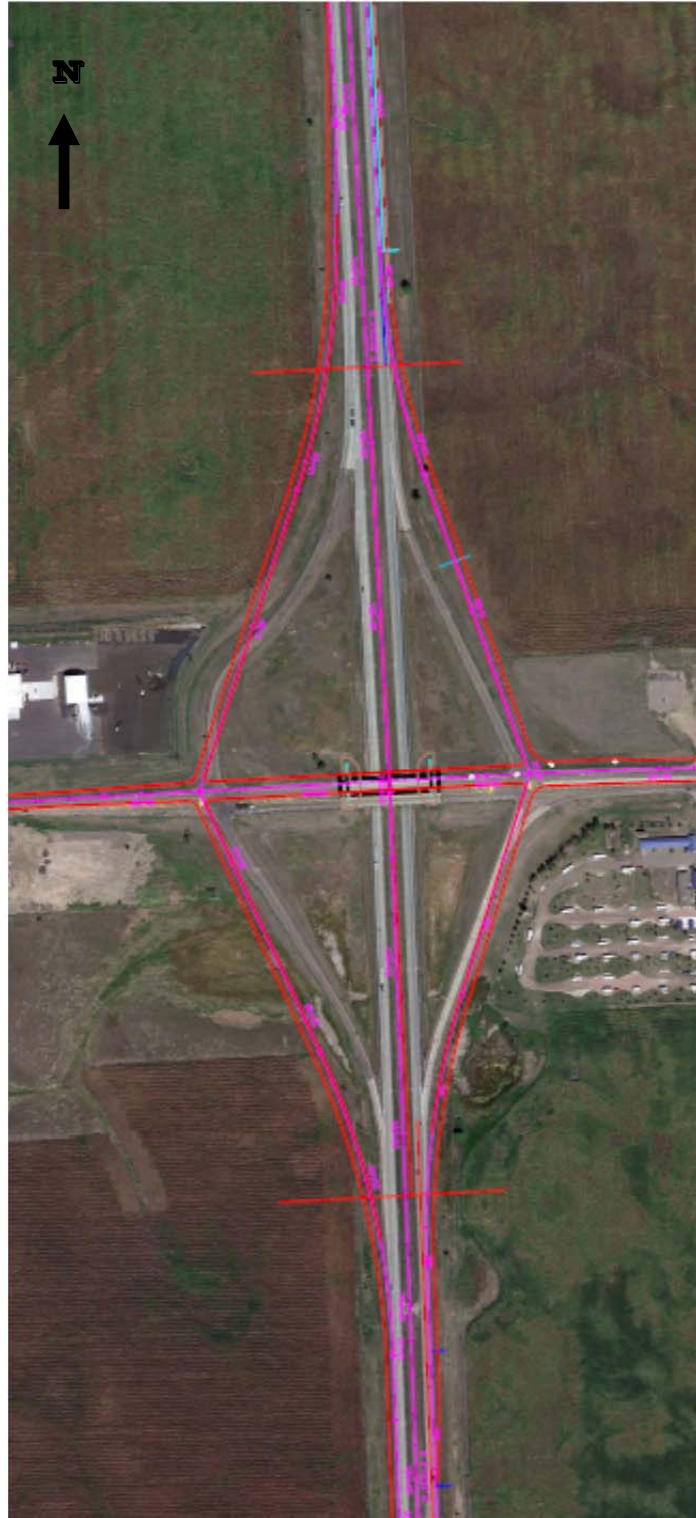
Figure 10: Alternative 1 – Diamond Interchange Configuration
