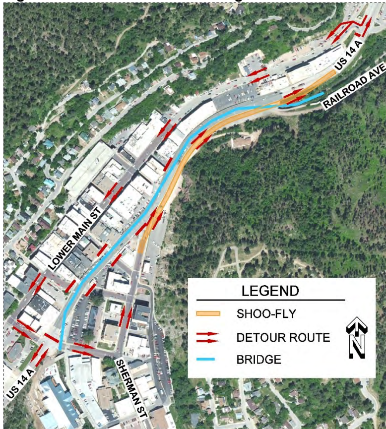
Figure 16.5 Traffic Detour during Construction
