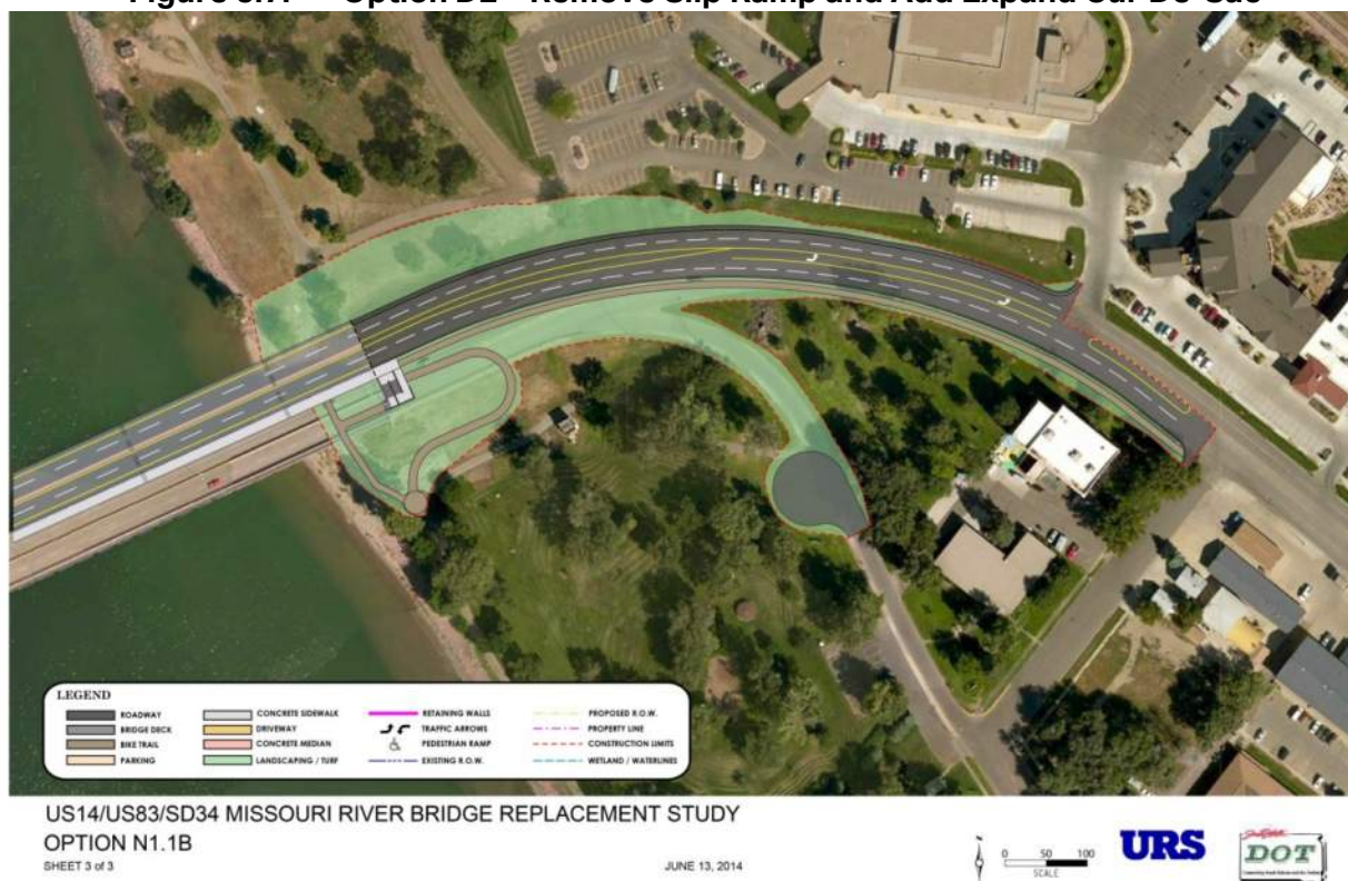
Figure 5.7: Option D2 – Remove Slip Ramp and Add Expand Cul-De-Sac
