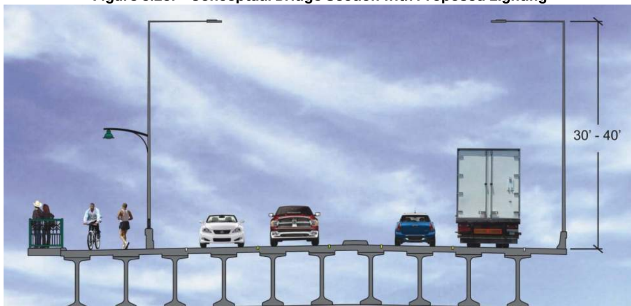
Figure 5.29: Conceptual Bridge Section with Proposed Lighting
