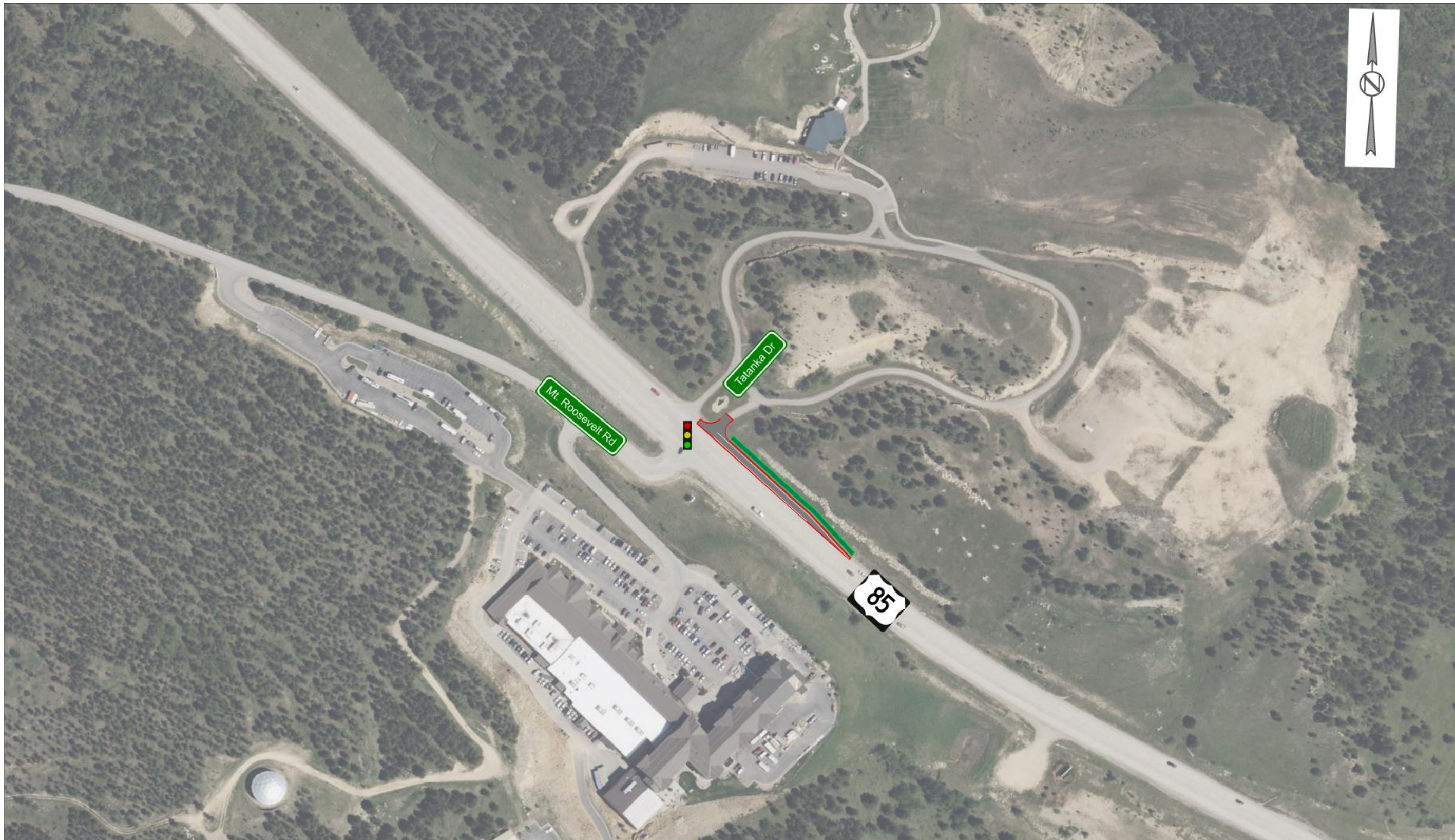
Figure 37: Alternative G2 – Signalization (with northbound right-turn lane)
