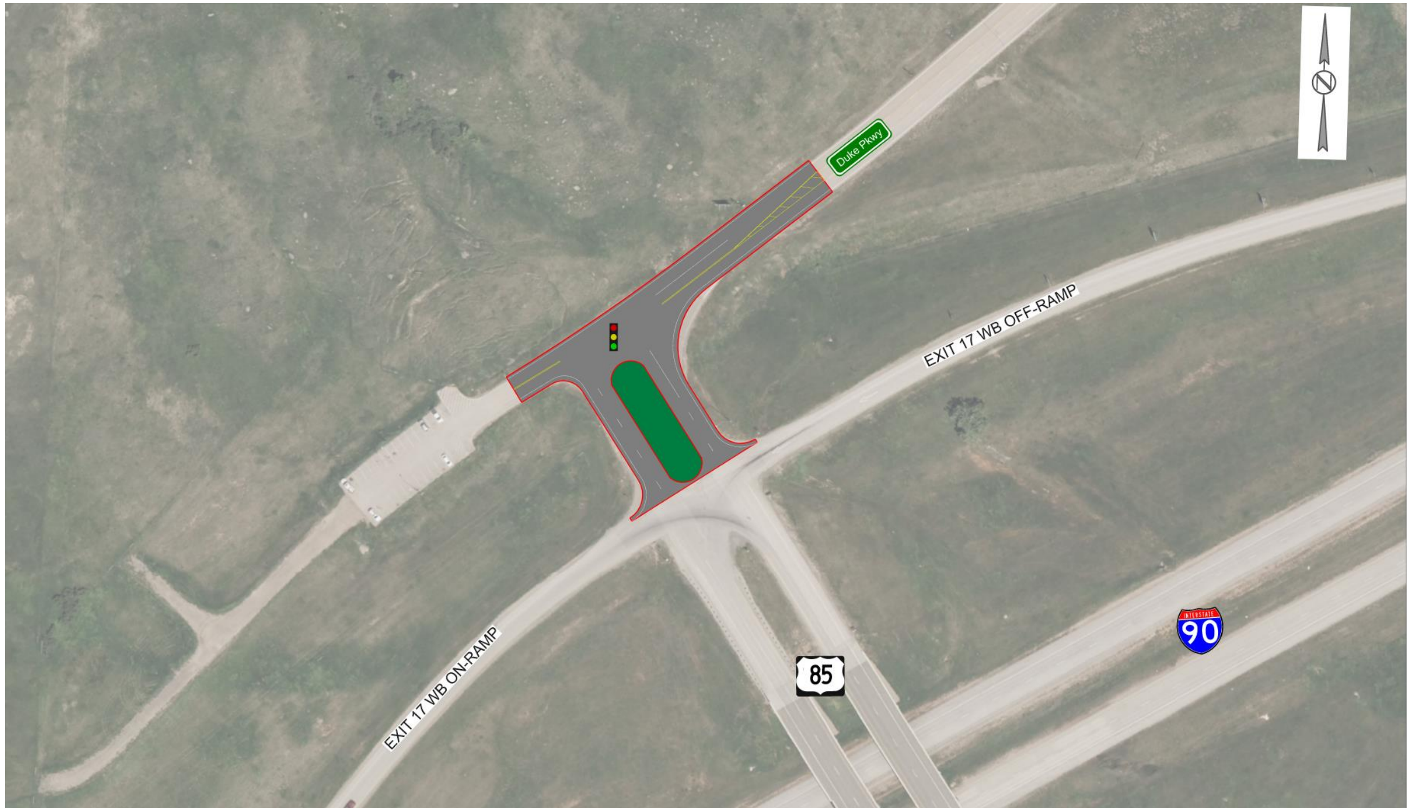
Figure 14: Alternative A2 – Signalization with Northbound Left-turn Lane
