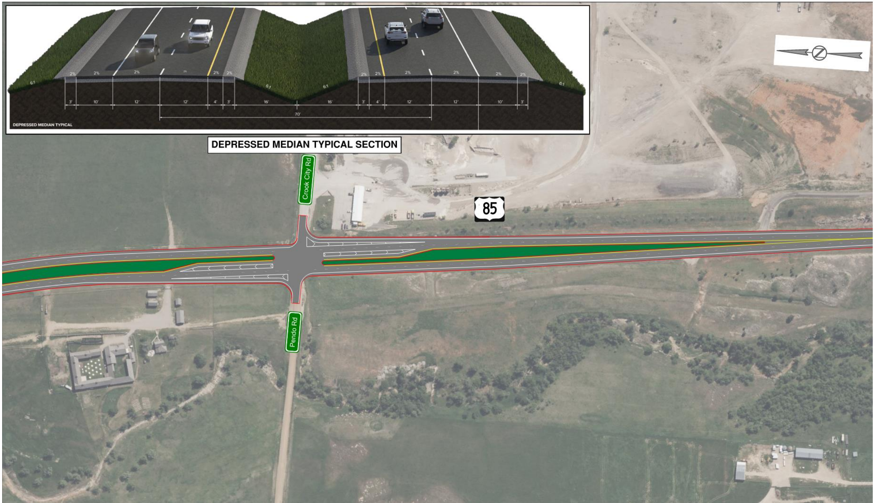
Figure 45: Alternative I1 – Extend Existing Typical Section to Crook City Road/Pendo Road
