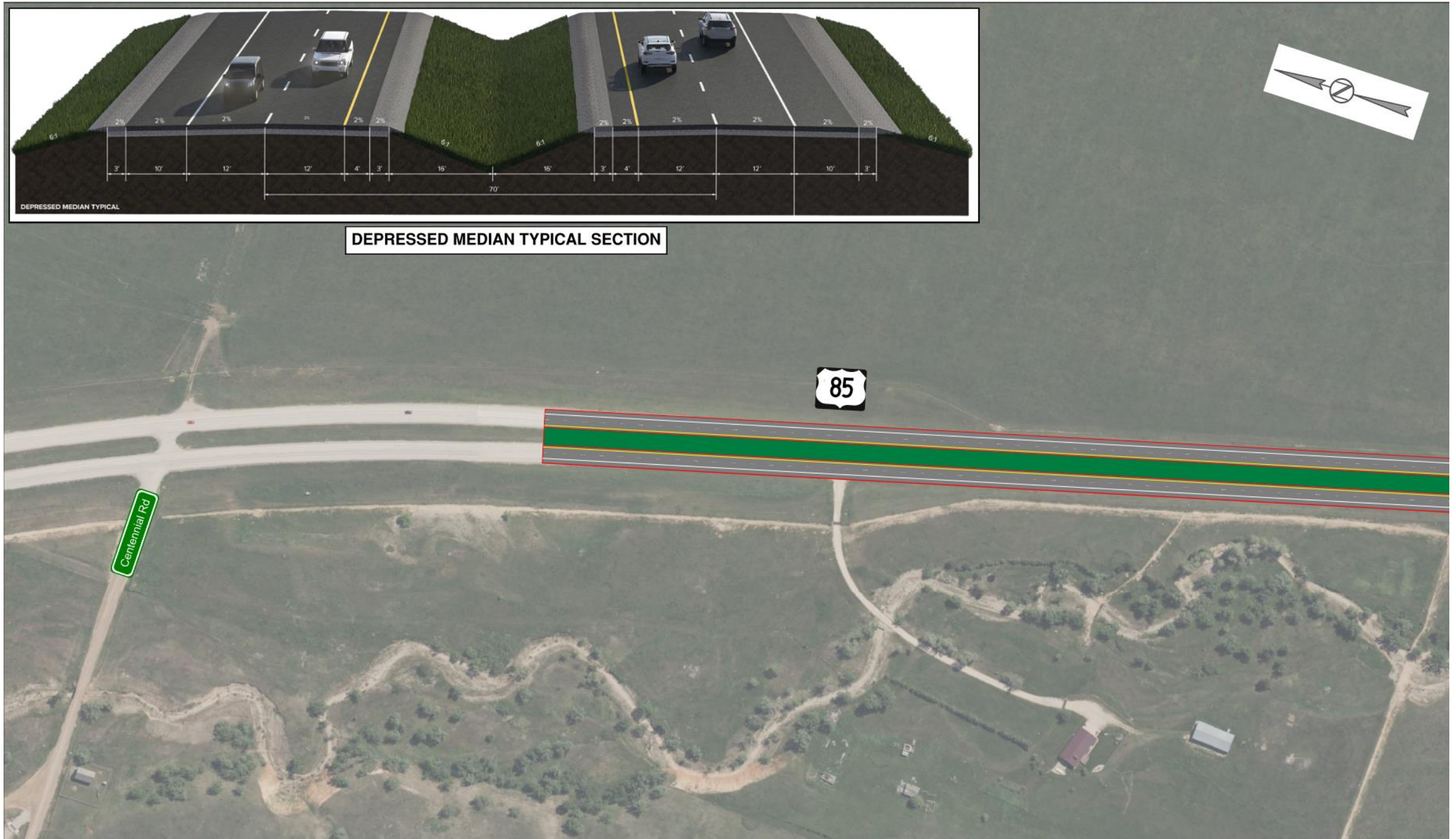
Figure 44: Alternative I1 – Extend Existing Typical Section to Crook City Road/Pendo Road
