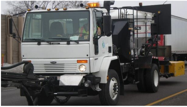
Step 1. A blow patch truck.
