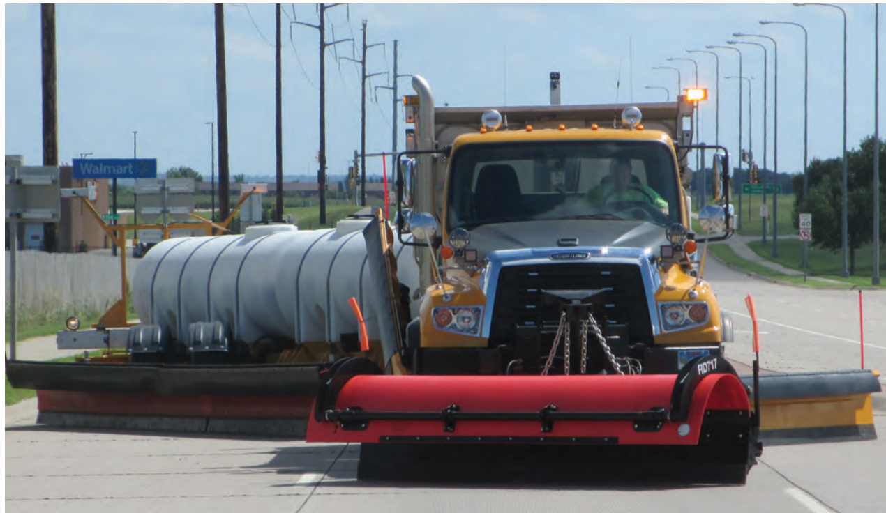
An SDDOT snowplow driver in the Sioux Falls Area practices pulling the new tow plow . The white tank holds salt brine, which is used to prevent ice formation.
