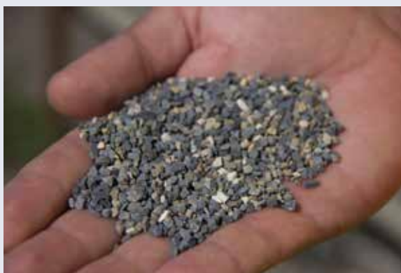
Calcined bauxite aggregate used for high-friction surface treatments
