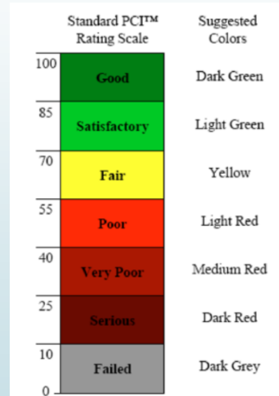
FIG. 1 Pavement Condition Index (PCI), Rating Scale, and Suggested Colors
